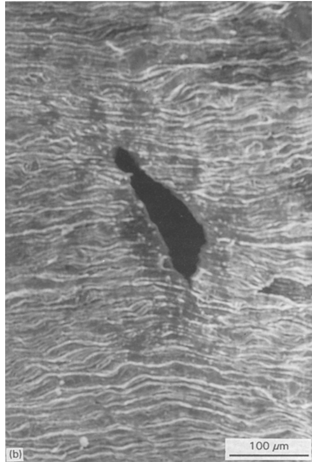
Figure 13 (a) Grain elongation and the formation of separate rounded cavities in the necked region of a B_L specimen; \dot{\epsilon}_0 = 2.7 \times 10^{-4} \text{ s}^{-1} ; elongation at fracture 387%; (b) a B_T specimen tested at the same \dot{\epsilon}_0 ; an elongated cavity, with its major axis nearly perpendicular to the stress axis is seen; elongation at fracture 381%. (c) Interior (nearly equiaxed) grains seen through the surface cavity in (b).
